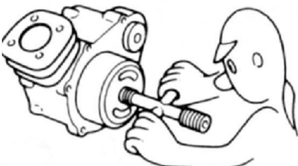
■ If the disassembling of pressed ball bearing is done by pressing the balls, the disassembled should not be used again.
