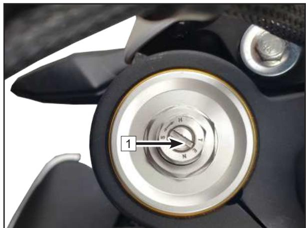
Use a flat-head screwdriver to rotate the gear counterclockwise (S direction) and record the times to reduce the recovery damping. Use a flat-head screwdriver to rotate the gear clockwise (H direction) and record the times to increase the recovery damping.
