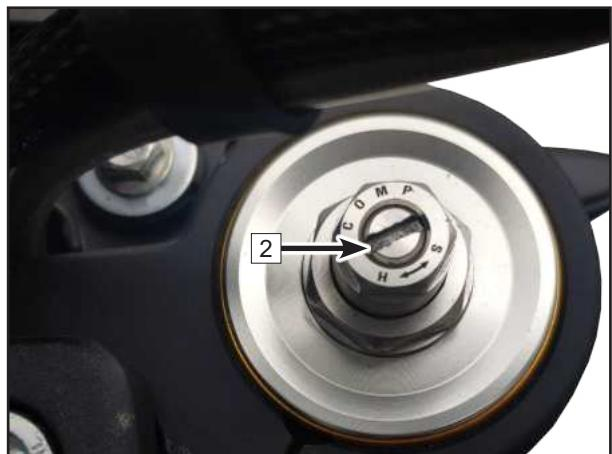
and record the times to increase the compression damping.
