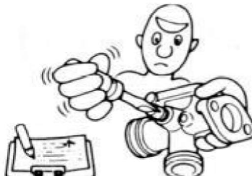
■ If not know the length of screws, install the screws one by one and tighten with same torque.
