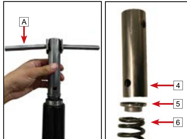
Retrieve and hold the damping rod to prevent it from dropping.
