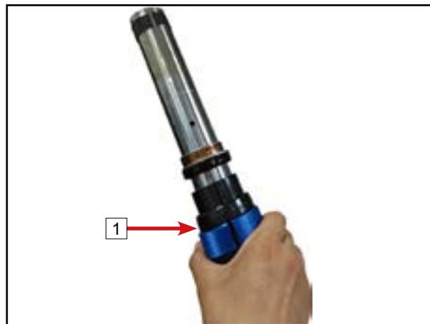
Insert the inner tube into the outer tube **2**. Then strike the oil seal with the oil seal impact tool **1** until the oil seal is firmly pressed into the outer tube and the groove for the retaining ring is visible.
