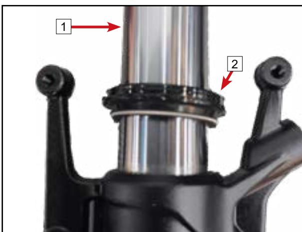
Dislodge the retaining ring **3** using a plastic blade or another appropriate tool. Press this tool firmly against the ring, and gently pry. Avoid scratching the inner tube while dislodging the ring.
