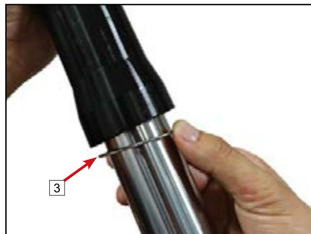
Install the dust boot **4** by hand. Its lip should sit flush with the outer tube end.
