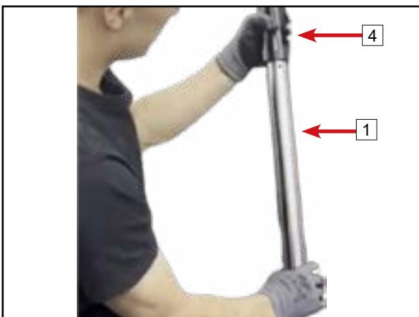
Remove the guide bushing set **d**, oil seal **c**, retaining ring **b** and dust boot **a** from the inner tube. Record the removal sequence for future reference.
