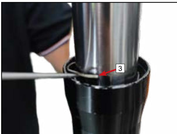
Tightly hold the outer tube **4** with one hand and the inner tube **1** with the other hand. Jerk the outer tube upwards until the inner tube separates from the outer tube.
