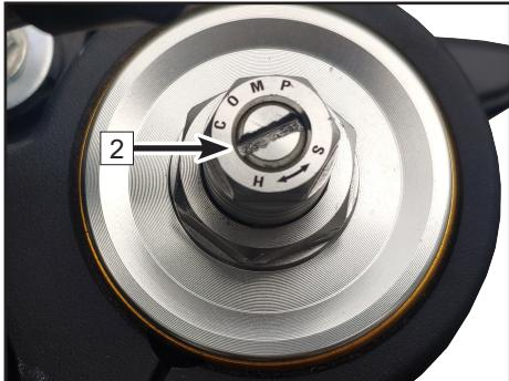
Rotate the adjuster counter-clockwise (S direction) by straight screwdriver and record the number to decrease compression damping. Rotate clockwise (H direction) by straight screwdriver and record the number to increase compression damping.
